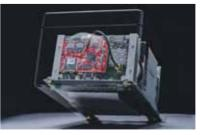
or Digital I/Os) linking up to 300 different environmental sensors to one data-logger. Data from these sensors can trigger alarms and operate switches; other sensors and gauges.
