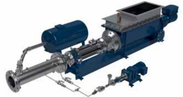
force has been overcome, the sludge plug is moved by pulsed controlled compressed air, which again reduces the discharge pressure in the pipework. Adjusting system parameters, such as polymer and air volumes, makes it possible to set a plant-specific, energy-optimised operating point.
