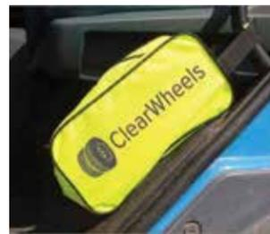
The ClearWheels System comprises of a chain with webbing strap at either end that the driver feeds behind the foreign object and back out again. The straps are then placed in front of the leading wheels, or behind the trailing ones, then either drives forward or reverses back depending on which set of wheels the debris is stuck between.
