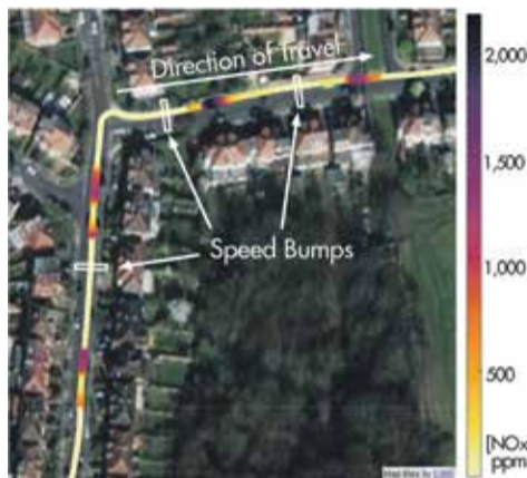
Effects of speed bumps on NOx emissions in West London urban environment
