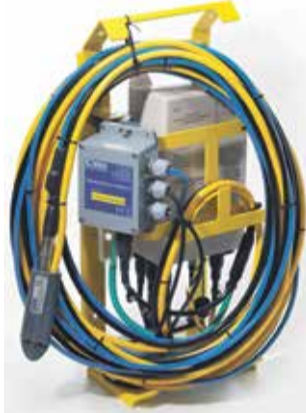
Pass Forward Flow (PFF) monitoring and final effluent monitoring.
