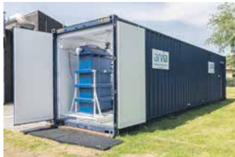
Containerised plug and play Nyex™ system
