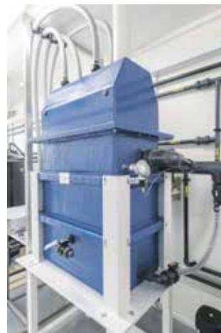
Nyex™ 16-50e reactor tank
