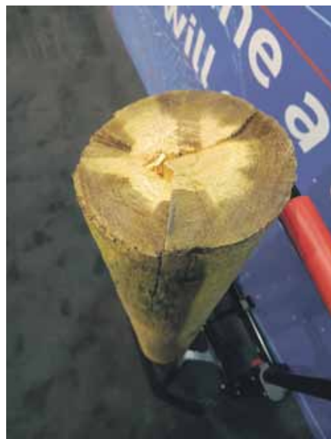
Typical problem with pressure treated poles
