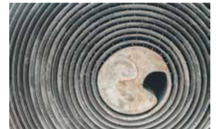
Spiral heat exchangers are difficult to clean and service
